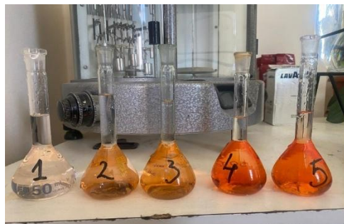
Figure 6. Standard solutions with increasing concentrations of \text{Fe}^{2+} (0–1.5 mg/
