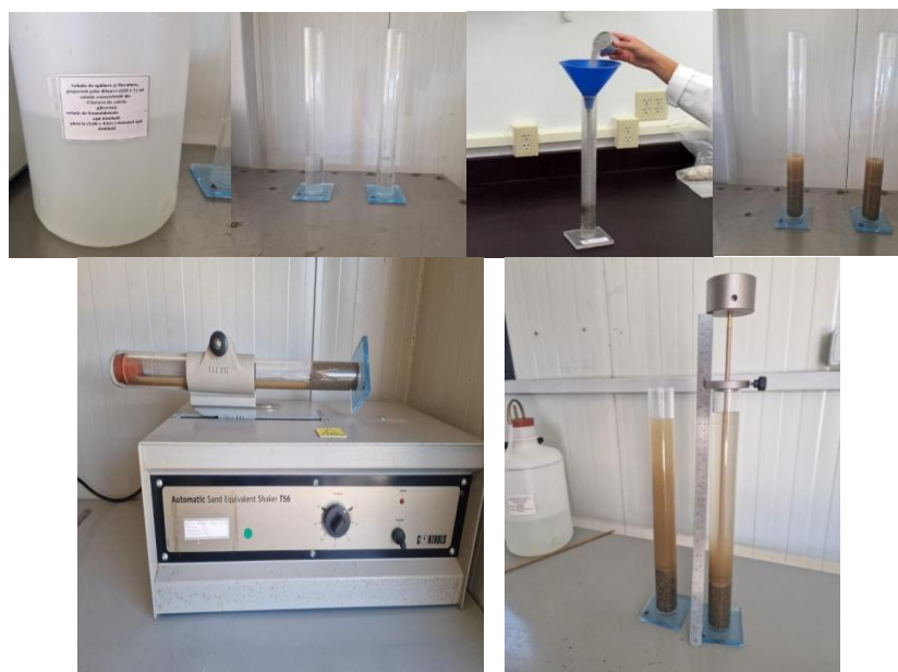
Figure 5. Sand Equivalent Test Steps
