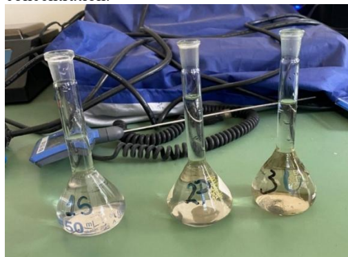
Figure 7. Mineralized samples completed at 50 mL, prepared for iron content analysis.
