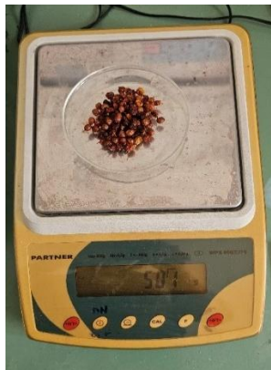
Figure 3. Weighing of Dried Sea Buckthorn Fruit Solid Sample for Extract Preparation
