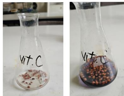
Figure 6. Sea buckthorn dried fruit extracts before and after determination of vitamin c concentration by titration with \text{KIO}_3 0.001 N in the presence of starch
