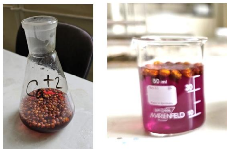
Figure 5. Sea buckthorn extract solutions before and after titration with 0.01 M EDTA in the presence of murexid for calcium determination
