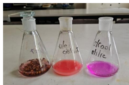
Figure 9. Sea buckthorn samples after determination of acidity with NaOH 0.1 N in the presence of phenolphthalein: aqueous extract of dried sea buckthorn fruits; extract in ethyl alcohol of volatile sea buckthorn oil; control sample of ethyl alcohol
