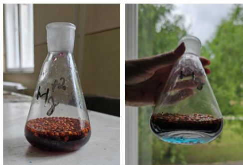
Figure 4. Samples of aqueous extract of dried sea buckthorn fruits before and after titration with EDTA 0.01M at pH 10
